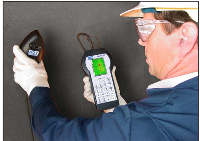
The Pocket UT's portability allows for quick, thorough mapping of areas where suspected corrosion may exist.
